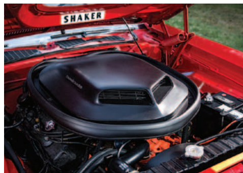
The Shaker hood setup included a cable control so the driver could manually open or close the scoop for maximum performance.
